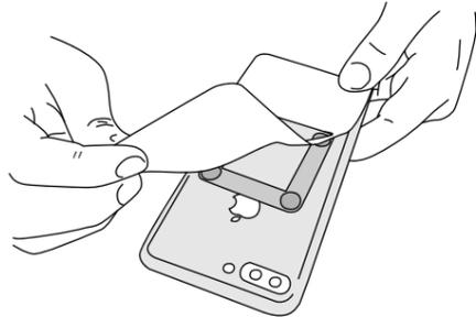
Once the template is placed, stick the Magnetic Patch in the hole of the template
