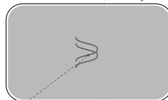
The W indicates the exact location of the wireless charging transmitting coil
